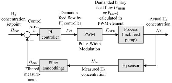
Figure 3. Block diagam of the H<sub>2</sub> concentration feedback control system.
