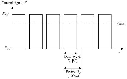
Figure 3. Pulse-Width Modulation (PWM), which is used to control the feed pump.
