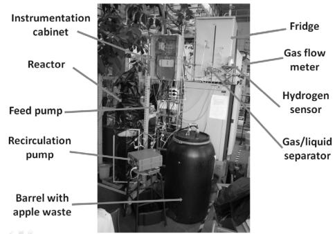
Figure 2. The biogas reactor.
