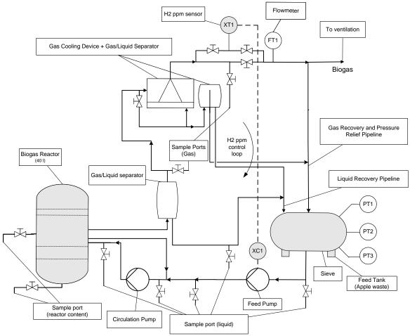
Figure 1. P&ID (Process and Instrumentation Diagram) of the biogas system.
